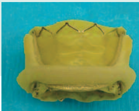
C - Bench test of 29 Sapien within a 29 Perimount 'side view'
